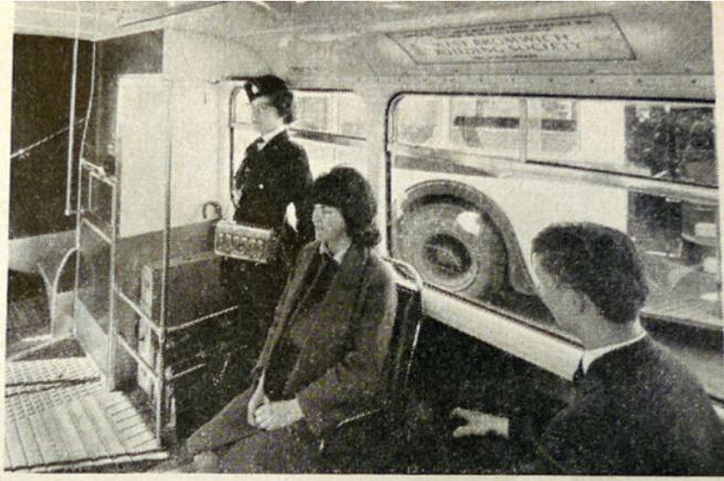
Part of the front end of the lower saloon on one of the 1963 deliveries of Titans with Weymann-built M.C.W. bodies. It shows the luggage space and the room given for the conductor to stand. The Perspex-covered fluorescent light fitting was manufactured to Bournemouth's specification.
